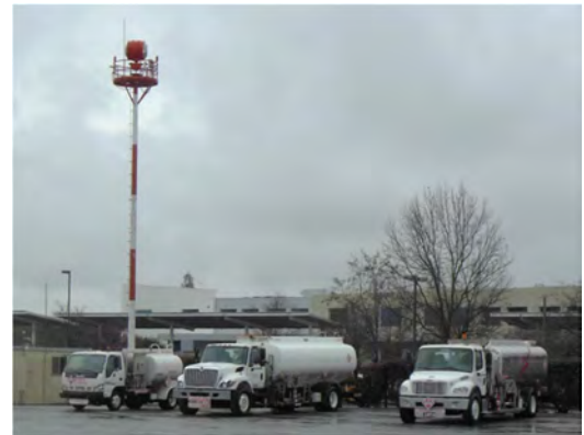
Airport Rotating Beacon and Mobile Refueling Trucks
